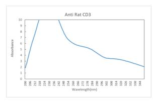
Description: 0.5 mg/mL Mouse anti rat CD3, protein type Mouse IgG3, containing protein stabilizer and sodium azide ( $\leq$  0.09%), measured by Nano-100 spectrophotometer, the concentration curve was abnormal, A280=5.195, which does not meet the labeled concentration.
