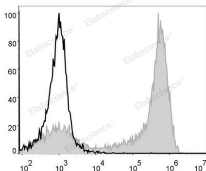
C57BL/6 murine bone marrow cells are stained with PE/Cyanine5 Anti-Mouse Ly6G Antibody (filled gray histogram). Unstained bone marrow cells (empty black histogram) are used as control.
