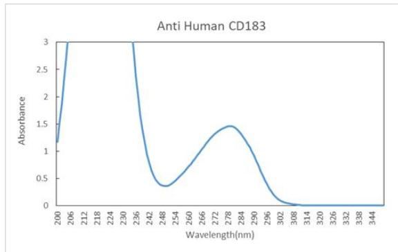
Description: 1 mg/mL Mouse anti human CD183, the protein type was Mouse IgG1, PBS (pH 7.2, no preservatives), measured by the Nano 100 spectrophotometer, the concentration curve was normal, and  $A_{280}=1.454$ , in line with the labeled concentration.
