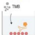
3. Add 90  $\mu$ L of Substrate Reagent. Incubate for about 15 min at 37°C
