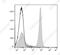
Staining of C57BL/6 murine splenocytes cells with PE/Cyanine7 Anti-Mouse CD45R (B220) Antibody[RA3-6B2] (filled gray histogram) or PE/Cyanine7 Rat IgG2a, κ Isotype Control (empty black histogram). Total viable cells were used for analysis.
