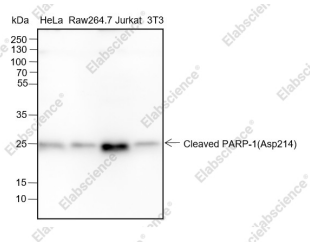
Western Blot with Cleaved PARP1 p25 Monoclonal Antibody at dilution of 1:2000. Lane 1: HeLa, Lane 2: Raw264.7, Lane 3: Jurkat, Lane 4: 3T3
